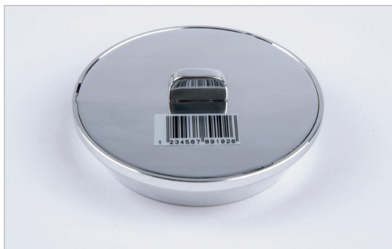
Each filter during conditioning is stored in a steel container.
