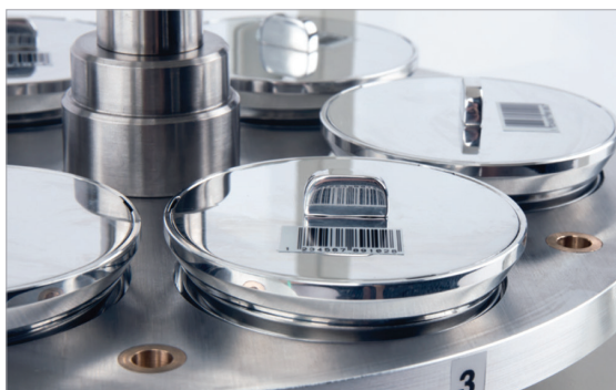
The filters are identified by a number being a combination of a digit code of a magazine position and EAN code of the weighing container (option).
