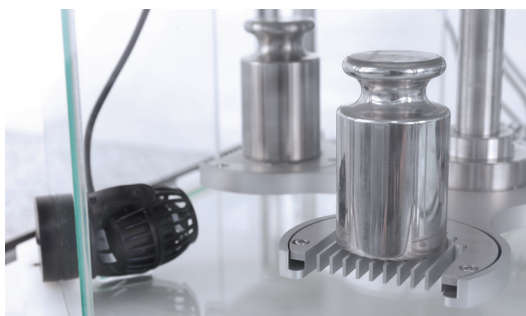
The device is equipped with an additional circulator eliminating air bubbles which may occur while loading the magazine with a mass standard.
