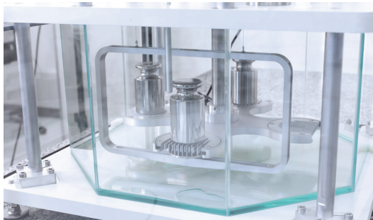
A weighing pan suspended on wires of 0.3 mm diameter significantly minimizes the eccentricity and the influence of liquid surface tension.
