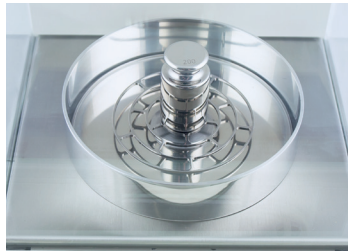
Openwork weighing pan significantly reduces ambient conditions influence on the measurement.
