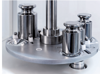
Extraordinary design of the weighing pan enables both, comparison of mass being combination of 3 weights, and standard comparison of 1 weight.
