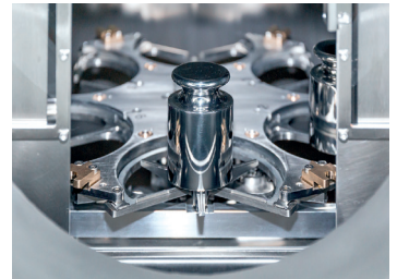
Suspended weighing pan of custom design eliminates eccentricity errors and facilitates dropping the weight onto the magazine insert correctly.
