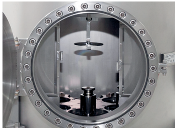
Used chamber enables comparison in vacuum of maximum 10 (-6) mBar or in noble gases such as argon.
