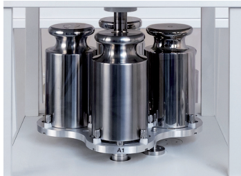
Weight positioning of sliding nature prevents errors of eccentricity.
