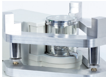
The modular design enables to use the susceptometer as a microbalance or a mass comparator.
