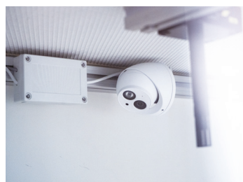
Remote preview of comparison process in real time is possible thanks to a video camera.
