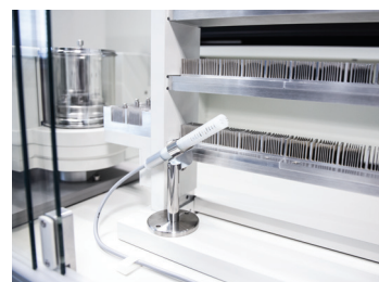
The mass comparator allows real-time monitoring of ambient conditions.
