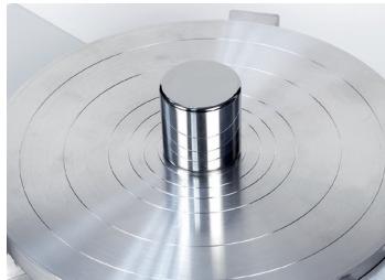
Positioners on the susceptometer weighing pan facilitate centring of the mass standard.
