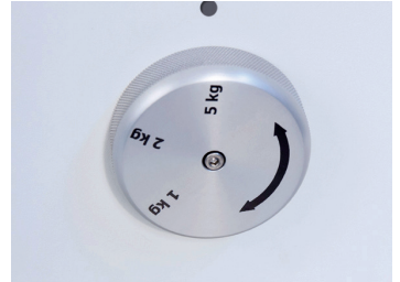
Weighing range switch allows you to select different load ranges for weights comparison. Regardless of selected option, constant comparator resolution is maintained.
